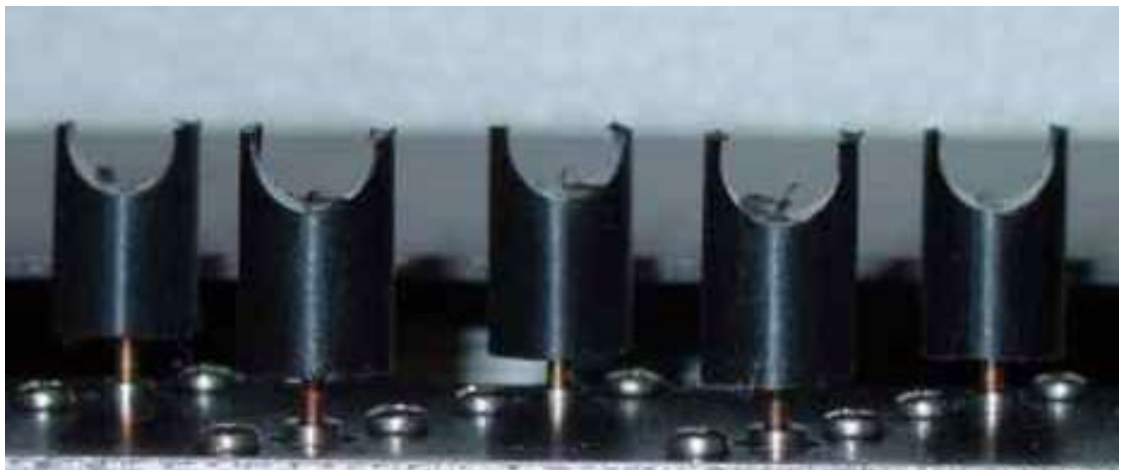
FIGURE 3-21 - SOLENOID TIPS ALIGNED CORRECTLY
